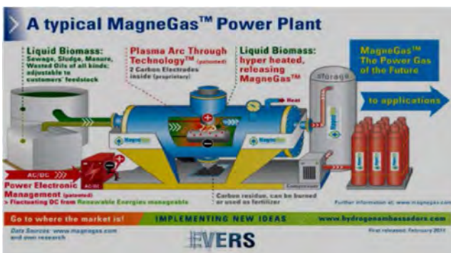
Figure 14. Future Scope II: Applications of MagneGas in Power Plant as future scope.
