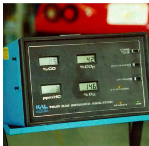
Figure 11. A picture of the readings of a 4-ways exhaust analyzer testing the exhaust of the Ferrari 308 GTSi of a preceding picture operating on magnegas "without" catalytic converter. Note: the presence of 14% breathable oxygen in the exhaust; about half the CO 2 produced by the same car when running on gasoline; the very few detected hydrocarbons originate from engine oil seeping through the piston rings because magnegas cannot contain hydrocarbons since it is synthesized at the 5, 000°C of the arc at which temperature no hydrocarbon can survive; the very small content of CO in the exhaust is due to poor combustion because CO is fuel for magnegas, while it is a byproduct of the combustion for fossil fuels, as a result of which detecting CO in the exhaust of a car running on magnegas is the same as detecting gasoline in the exhaust of a car running on gasoline.
