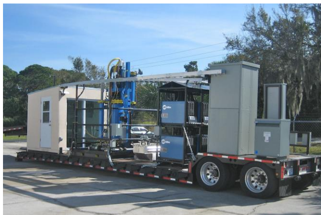
Fig. 4. view of the gasifiers built by the author when Chief Scientist of Magnegas Corporation converting liquids into the clean burning magnegas fuel.
