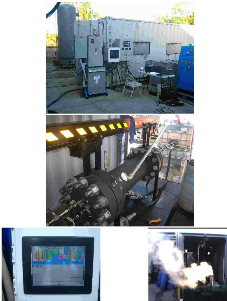
Figure 28: A view the Hadronic Reactor III built and used by the author for the synthesis of Silicon from Carbon and Oxygen, the synthesis of Titanium from Silicon and oxygen and other ICNS [110-120] (see Ref. [114] for a video on the reactor and ref. [115] for its sound during operation).
