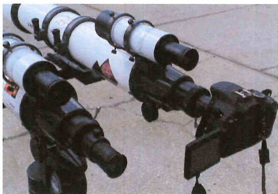
Figure 16. A close up view of the mounting of the camera directly in the telescope in place of the eyepieces [43].
