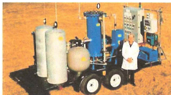
Figure 9. Picture of a 50 kW Santilli's Hadronic Reactor (Plasma Arc Flow Recycler) mounted on a trailer for mobility to conduct test recycling where liquid wastes are located. This recycler can produce up to 84, 000 scf (up to 2.4 million liters) of magnegas per week corresponding to about 560 gasoline gallon equivalent (2, 100 gasoline liter equivalent) of magnegas per week.
