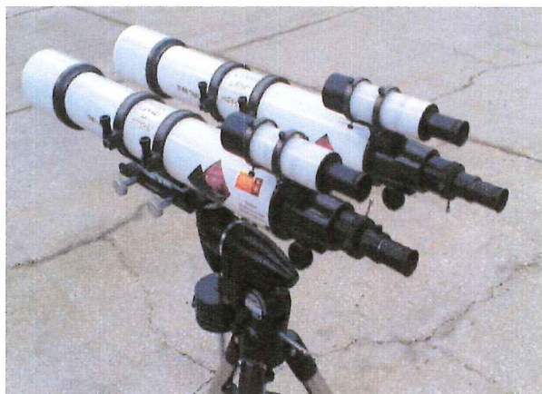
Figure 15. The parallel mount of the Galileo and antimatter telescopes with related finder scopes [43].
