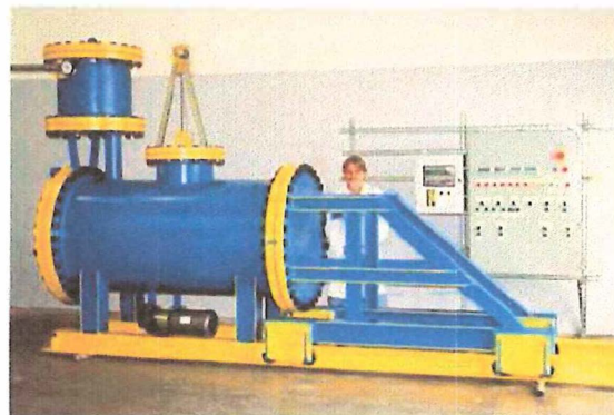
Figure 8. Picture of a 250 kW Santilli's Hadronic Reactor [3] (also called Plasma Arc Flow Reactor) with the panels of its completely automatic and remote controls, to recycle liquid waste into magnegas usable for any fuel application, a large amount of heat and carbonaceous precipitates used to produce the electrodes. This Reactor can produce up to 5000,000 scf (140 million liters) of magnegas per week of 24 hours work per day corresponding to 3,000 gasoline gallon equivalent (11,000 gasoline liter equivalent) of magnegas per week.
