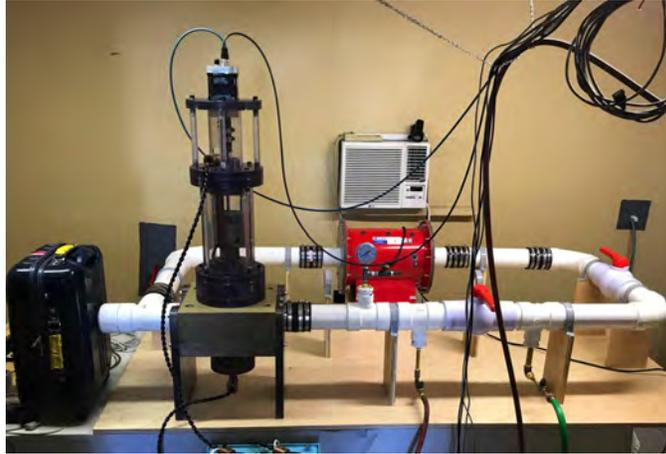
Figure 12: A view of the *Directional Neutron Source (DNS)* described in Section 8.2.4 which synthesizes on demand neutrons from the hydrogen in the desired direction, flux and energy.
