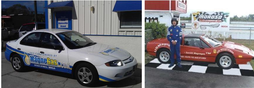
Figure 25: A view in the left of a Ford Cavalier produced to run on compressed natural gas and run on compressed magnegas with no appreciable CO and HC in the exhaust, and a view in the right of a Ferrari 308 GTS 1981 converted to run on compressed magnegas and shown at the Moroso International Race Track, Florida, to be competitive with same Ferraris running on gasoline.
