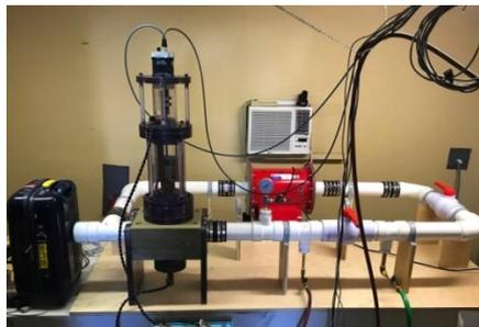
Fig. 12. A picture of the "Directional Neutron Source" (DNS) based on the laboratory synthesis of the neutron from the hydrogen which is in production and sale by Thunder Energies Corporation [46] for the detection of fissionable material that may be concealed in suitcases.
