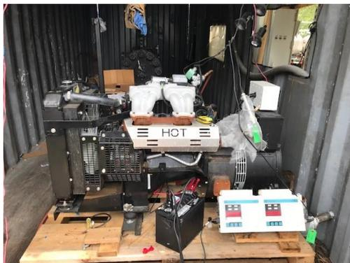
Fig. 16. A picture of the 12 kW General Motor Electric generator (GMEG) used for the experimental verification of the pseudoproton reported in this paper for the first time.
