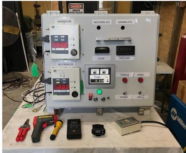
Fig. 14. A picture of a remote monitoring and control station of the DNS of Fig. 12.
