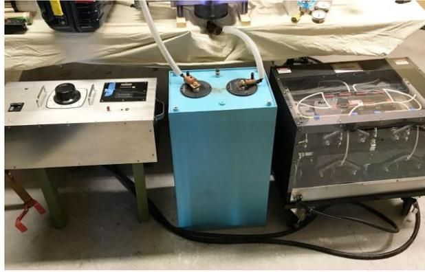
Fig. 13. A picture of the power unit and capacitor of the DNS of Fig. 12.
