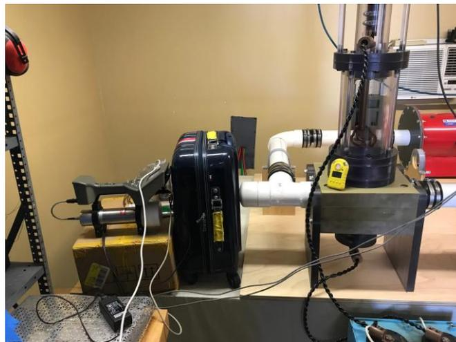
Fig. 15. A picture of detectors capturing the radiation emitted by fissionable material that may be contained in a suitcase when irradiated by a neutron flux.
