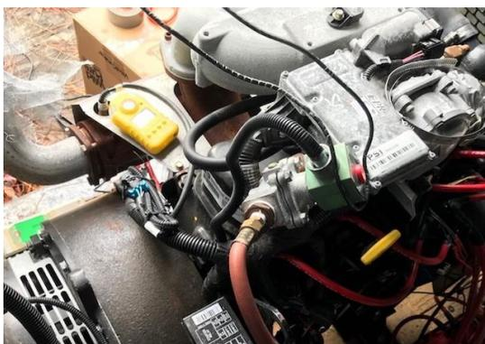
Fig. 17. A picture of the sole feeding of the GMEG of Fig. 16 via a hydrogen gas with a sealed air intake Fig. 18.
