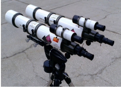
Figure 15: The parallel mount of the Galileo and antimatter telescopes with related finder scopes [43].
