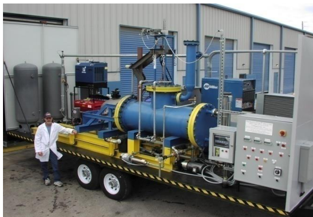
Figure 6 Picture of a 50 kW Santilli's Hadronic Reactor (Plasma Arc Flow Recycler™) mounted on a trailer for mobility to conduct test recycling where liquid wastes are located. This recycler can produce up to 84, 000 scf (up to 2.4 million liters) of magnegas per week corresponding to about 560 gasoline gallon equivalent (2,100 gasoline liter equivalent) of magnegas per week
