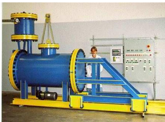
Figure 7 Picture of a 250 kW Santilli's Hadronic Reactor (also called Plasma Arc Flow Recycler™) with the panels of its completely automatic and remote controls, to recycle liquid waste into magnegas usable for any fuel application, a large amount of heat and carbonaceous precipitates used to produce the electrodes. This Reactor can produce up to 5000, 000 scf (140 millions liters) of magnegas per week of 24 hours work per day corresponding to 3, 000 gasoline gallon equivalent (11, 000 gasoline liter equivalent) of magnegas per week computed on the basis that: 1) Gasoline contains about 110, 000 BTU/g (about 29, 000 BTU/liter); 2) Magnegas has the low energy content of 750 BTU/scf (26 BTU/liter); and 3) the "gasoline gallon equivalent" is given by about 150 scf of magnegas ("gasoline liter equivalent" is given by about 29 liters of magnegas). Plasma Arc Flow Recycler™ are completely self-contained. Consequently, they release no solid, liquid or gas to the environment and cause no noise or odor pollution
