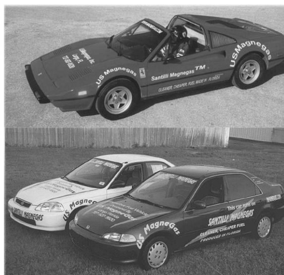
Figure 8 A picture of a Ferrari 308 GTSi 1980 and two Honda Civic cars converted by the author to operate with the new clean burning magnegas without catalytic converter, yet surpassing all EPA exhaust requirements, having no carcinogenic or other toxic substance in the exhaust, reducing of about 50% the CO 2 emission due to gasoline combustion, reducing the operating temperature of about 25%, and emitting in the exhaust 10% to 14% breathable oxygen
