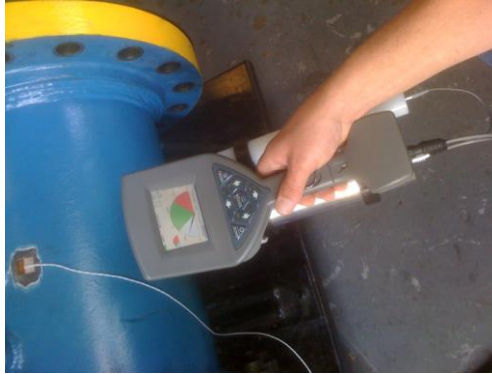
Figure 2. Photograph of PGT's model SAM940 gamma-ray and neutron detector
