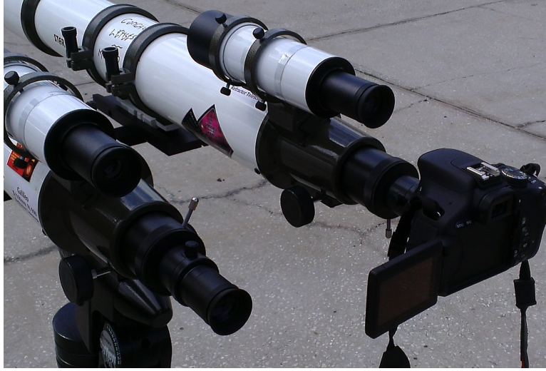
Fig. 5 A close up view of the mounting of the camera directly in the telescope in place of the eyepieces.
