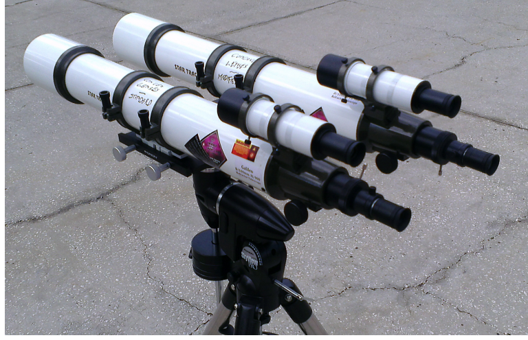
Fig. 4 The parallel mount of the Galileo and antimatter telescopes with related finder scopes.
